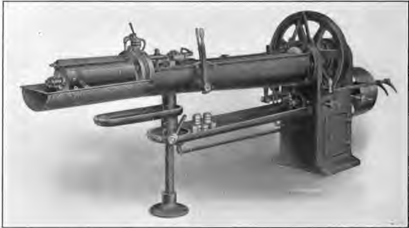
FIG. 60.—Broaching a core for an automobile hub.
